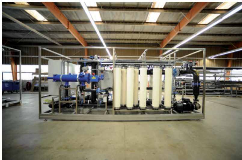
The Texel plant consists of an ultrafiltration membrane module treating 40 m 3 /h and a reverse osmosis unit.
